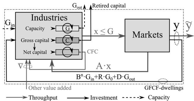
**Figure 3** Definition of the input-output system. The system drawing contains the most central system variables listed in table 1. Capacity, gross capital, and net capital are three aspects of industrial assets or fixed capital. They are accounted for in parallel.
