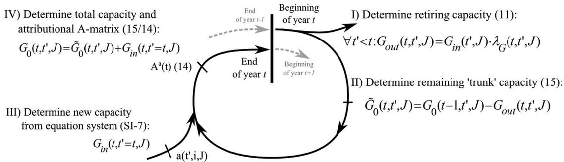
**Figure 4** Scheme of calculations for the year-by-year loop. Equation numbers are shown in brackets.
