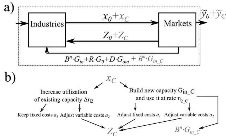
**Figure 5** (a) Original state (black) and perturbations (gray) of an industrial system after an increase in final demand. (b) The split of the additional output  $x_C$  into existing and new capacities and the resulting interindustrial flows  $Z_C$ .
